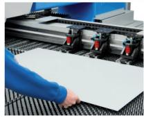
Manual loading is still possible to speed up production of small parts or batches.
