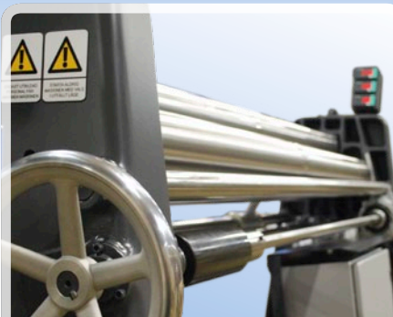
Cone bending equipment, includes diagonal setting of bending roll, trailing shoe and handwheel with dial register
