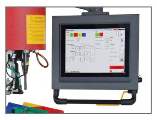
Operator control pendant can be adjusted in 6 directions.
