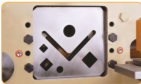
Ø and ∇ cut without deformation
