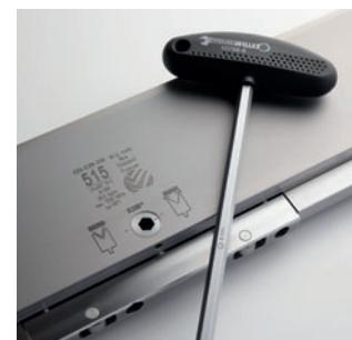
E2M® bottom tools are provided with an internal lift system. This system is applicable for a tool weight with a maximum of 140 kg /309 lbs and minimum tool length of 200mm/7.874". Minimum width of the tool should be 30mm/1.181".
