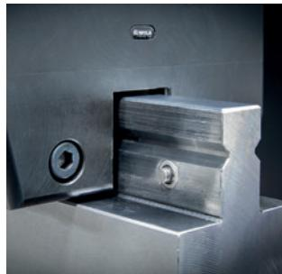
E2M® top tools are provided with bearing safety pins in the adaption of the tool. Applicable for: head and shoulder load top tools with a minimum tool length of 100mm/3.397". Tool weight should be between 12.5kg/28lbs and 100kg/220lbs.
