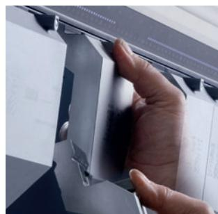
The Safety-Click® is WILA's patented safety mechanism which has been integrated into top tools with a weight up to 12.5 kg/28 lbs. This revolutionary mechanism allows tools to be changed vertically by simply clicking them in and out of the Clamping.
