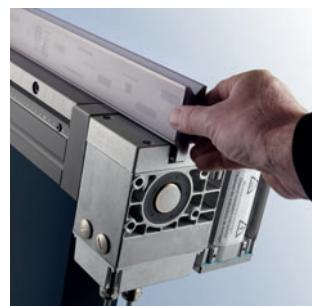
CRM7 is a CNC-driven drive motor which has been designed for New Standard Pro Crowning. This motor makes it possible to horizontally insert and remove bottom tools from both ends. The CRM7 motor is available for crowning lengths up to 4300 mm/14 ft.
