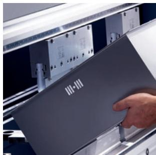
Extenders are used between the press brake's upper Clamping (or Tool Holder) and the top tool. Often they are used to heighten the top configuration, making it possible to bend deep boxes. These extenders are supplied as modules in lengths of 150 mm/5.91" and 515 mm/20.28". They are produced with extremely high precision, guaranteeing their interchangeability.
