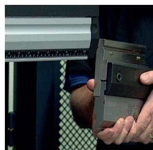
Adapters are used between the press brake's Clamping (or Tool Holder) and the top tool. Often they are used as an accessory to make the transition from one tool system to another. These adapters are supplied as modules in lengths of 150 mm/5.91" and 515 mm/20.28". They are produced with extremely high precision, guaranteeing their interchangeability.
