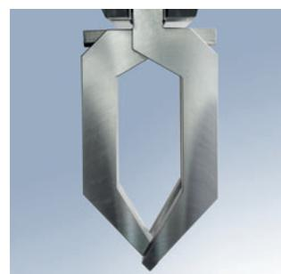
Because New Standard and American Style tools are symmetrical in relation to the centerline, these (top) tools can be easily rotated, such as when bending a reverse flange with a gooseneck tool.
