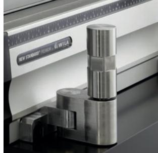
When using "HD" Tool Holders, it is possible to install 'pillars' to further support very wide and heavy bottom tools. These pillars offer additional stability to tools during the bending process. Available every 255 mm/10.039" on front and backside.
