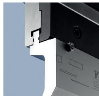
Within the framework of its UPB concept WILA has also included a mechanical clamping system in its program for American Style tools. This is a mechanical system in which the clamping is achieved by a continuous body with clamping plates. The top tools are clamped by manually tightening the clamping plates; the tools are not seated automatically. This mechanical system can be used for both the standard American Style top tools and the American Style top tools WILA re-designed with Safety-Click®.
