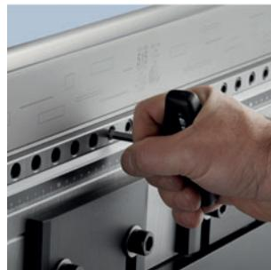
If bottom tool changeovers are not needed often, Premium and Pro Crowning/Bottom Tool Holder models with manual clamping are available as well. Manual Clamping is achieved via clamping bolts at a distance of every 25 mm/1", in the center 1.000 mm/40" and every 100 mm/4" towards each end, allowing the clamping of tool segments as small as 15 mm/0.591" in length.
