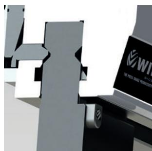
Tools are clamped using a pneumatically controlled pair of self-adjusting wedges. When the wedges are engaged (clamped), they become an integral part of the tool. This means tools always remain clamped, even if there is loss of air pressure. Clamping is also released pneumatically.
