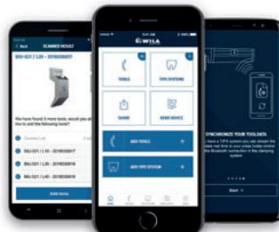
All WILA New Standard Premium tools have a unique DM-code. With the WILA Smart Tooling app you can scan all the tools. After scanning the DM-code you have immediate access to the tool's specifications and the correct tool data files for your press brake control.
