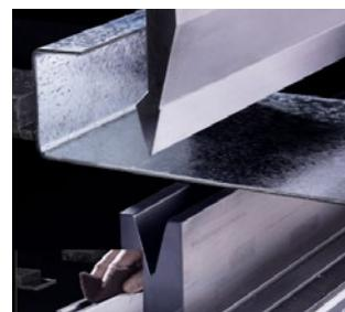
"Bending instead of cleaning!" OZU-ZN tools feature a coating that has been specially developed by WILA for use with galvanized material. This coating is applied to CNC-Deephardened® bottom tools and prevents zinc deposits from building on the bending radii.
