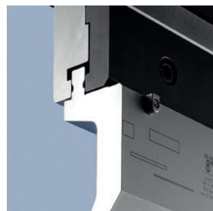
Within the framework of its UPB concept WILA has also included a mechanical clamping system in its program for American Style tools. This is a mechanical system in which the clamping is achieved by a continuous body with clamping plates. The top tools are clamped by manually tightening the clamping plates; the tools are not seated automatically. This mechanical system can be used for both the standard American Style top tools and the American Style top tools WILA re-designed with Safety-Click®.
