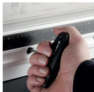
Ty-adjustment is crucial in achieving parallelism between top and bottom tools. Adjustment in Y direction makes it possible to fully compensate for unavoidable - cumulative - machining tolerances in the press brake. Either the top or bottom Tool Holder must be able to do this if one wants to achieve accurate and consistent bending results.
