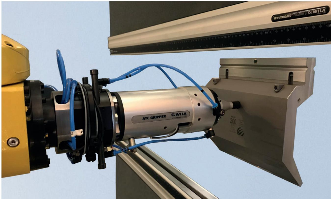
With automatic tool changes, the tool set-ups in your press brake are no longer the limiting factor in the variety of parts that can be formed entirely unmanned. The robot can change the part manipulator to the ATC Gripper, to be able to change tools quickly and efficient. The ATC Gripper can only handle special WILA ATC tooling (optionally executed with a TIPS ID-tag).
