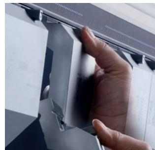
The Safety-Click® is WILA's patented safety mechanism which has been integrated into top tools with a weight up to 12.5 kg/28 lbs. This revolutionary mechanism allows tools to be changed vertically by simply clicking them in and out of the Clamping.
