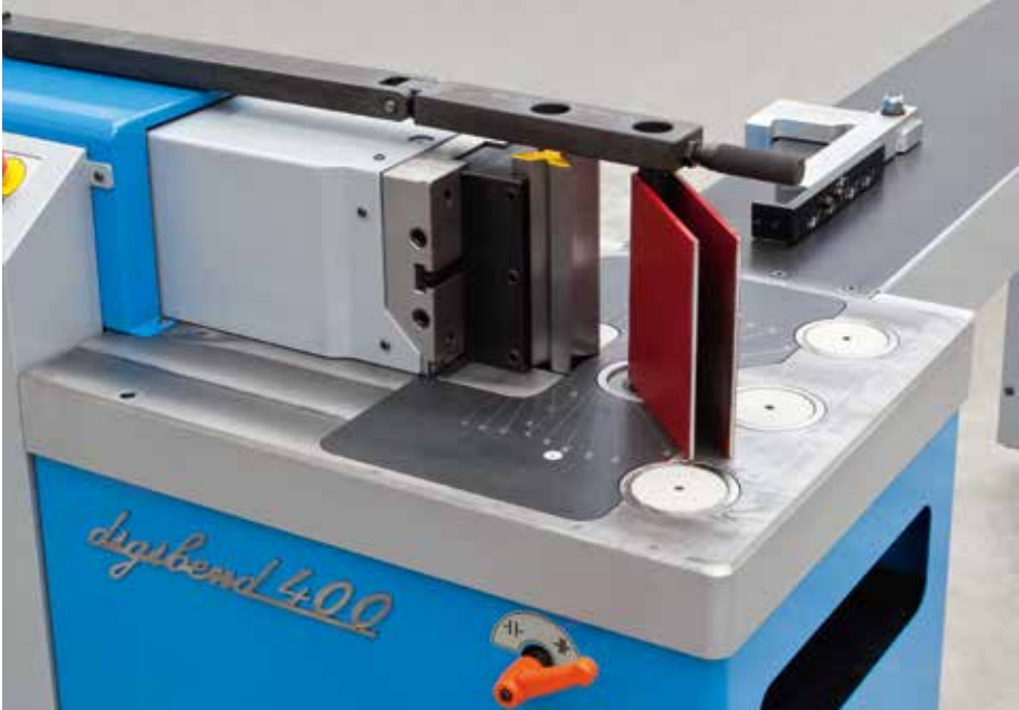
Bending tool with pin Ø 30 mm, H=200 mm and antiflection bar. Max 200 x 5 mm.
