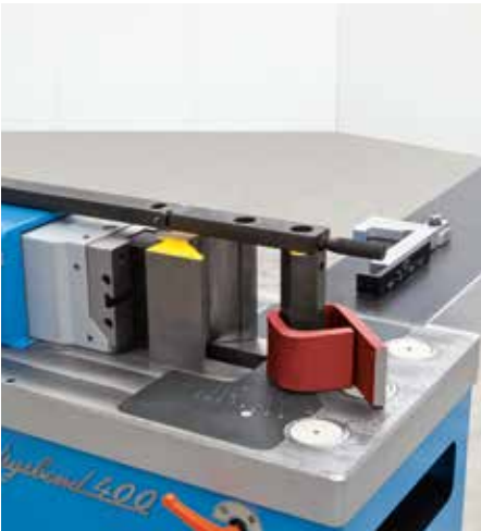
Pin bending punch Ø 80 mm with antiflection bar for bending a closed loop into thick wall bars. Max 200 x 15 mm.
