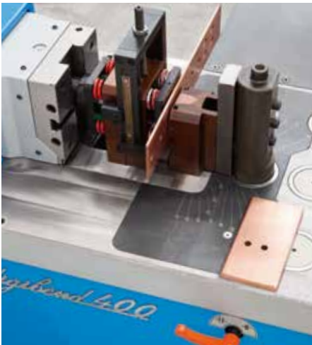
Punching unit for holes up to Ø 30 mm. Max thickness 12 mm.
