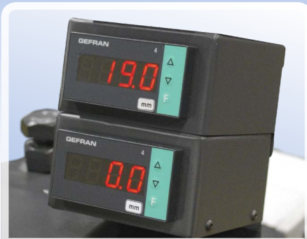
Digital display available for bending and/or lower rolls. Also available for feed length
