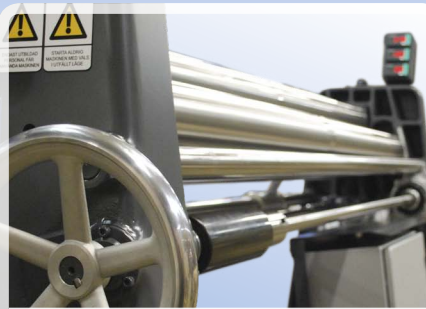
Cone bending equipment, includes diagonal setting of bending roll, trailing shoe and handwheel with dial register
